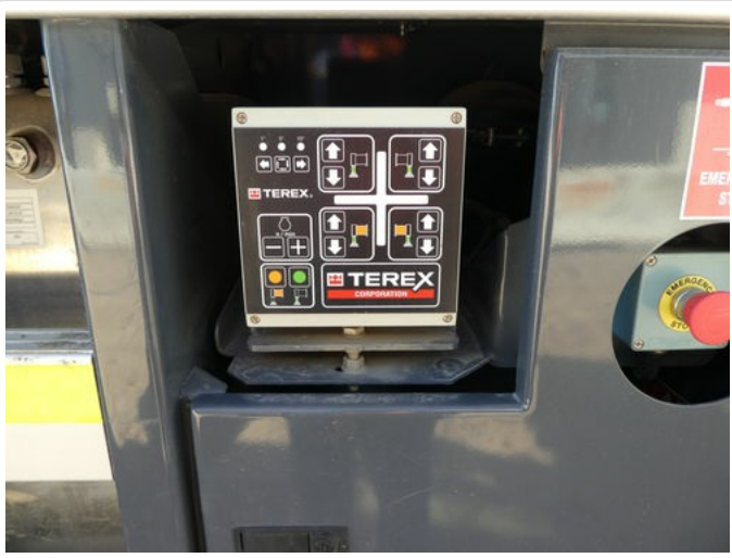
Outrigger Controls and Labeling outrigger controls and station levelling confirmed.
